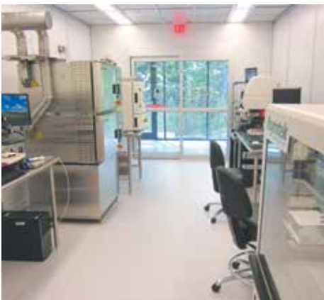
One of three ISO 6 (class 1000) cleanroom areas
